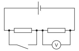
When the switch is open the voltmeter reads 1.5 V.
