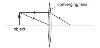
An image of the object is formed on a screen to the right of the lens.
